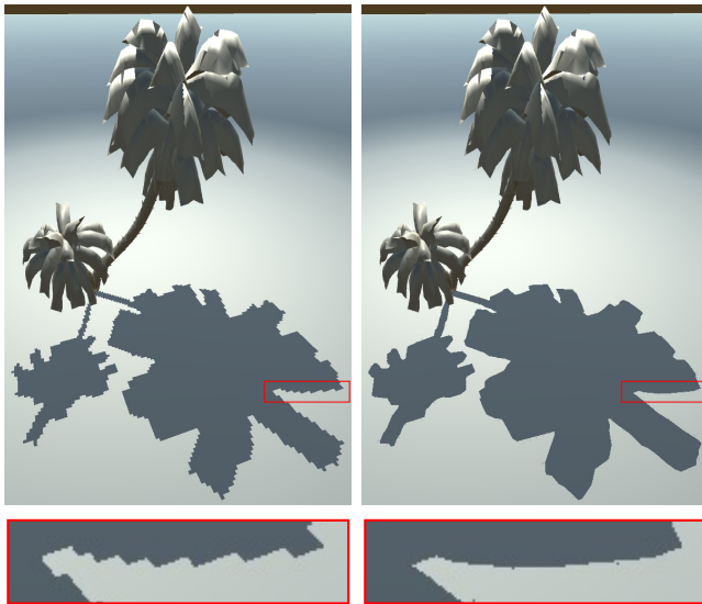
Figure 4: A visual comparison between shadow mapping (left) and RBSM (right) for the Coconut model using a medium-resolution ( 512^2 ) shadow map.
